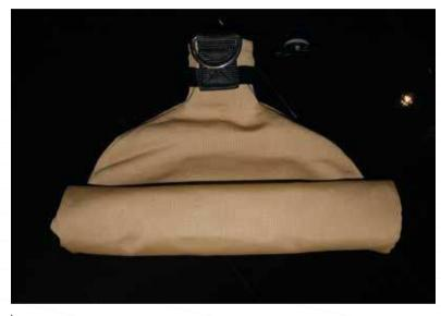
Deflate the fender. Close the inflation valve and the closure cap, making sure that no dust reduces its impermeability.
